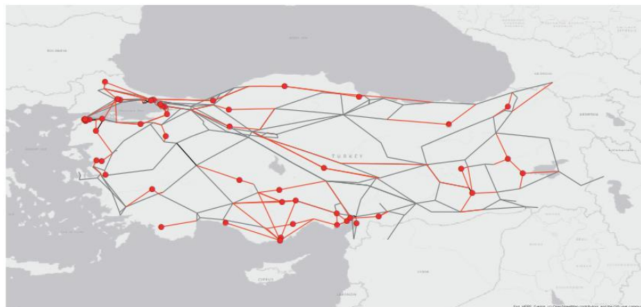
Figure 2: Map of current (grey lines) and planned (red lines and dots) 400-kV transmission grid as per the updated ten year (2021-2030) prospective network development plan
