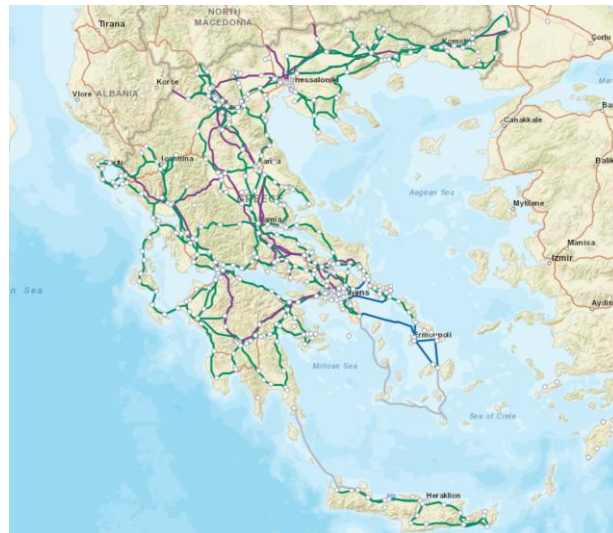
Figure 35. Current grid in Greece (purple lines 400 kV, green lines 150 kV, blue lines submarine cables)
