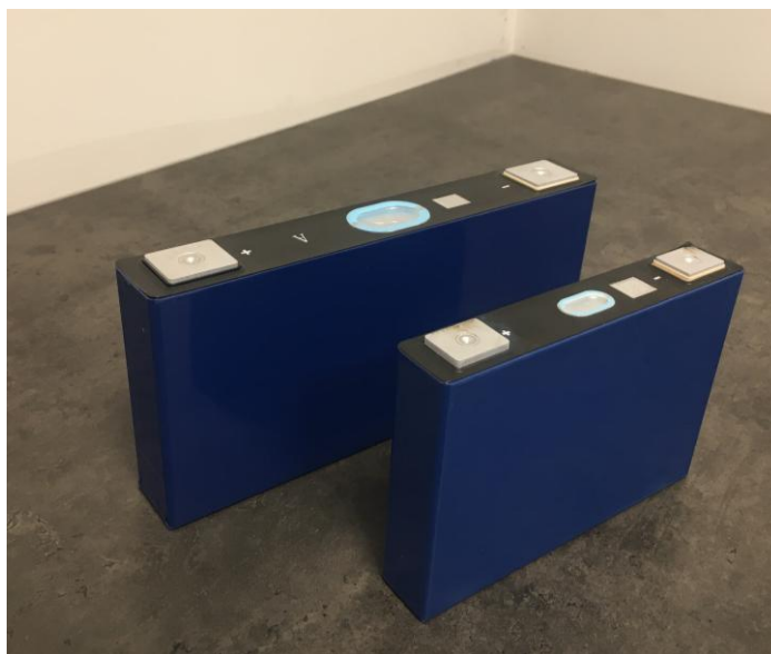
Figure 8: Comparison between NMC (right) and LFP (left) prismatic cells. While the capacity for LFP (113 Ah) is slightly less than two times the NMC (60 Ah), the volume is more than double.
